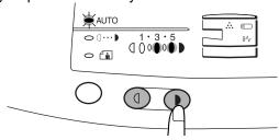
4 Press the exposure selector key. The AUTO indicator will stop blinking and light up steadily.
